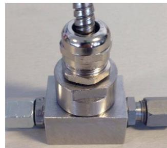
Fig.1 A photograph of the in-line viscosity sensor.
