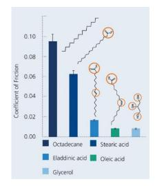
Fig.1 Superlubricity of self-mated ta-C coatings could be achieved with unsaturated oleic acid and glycerol. Saturated stearic acid has much lower reactivity and results in much higher friction common to boundary lubrication.
