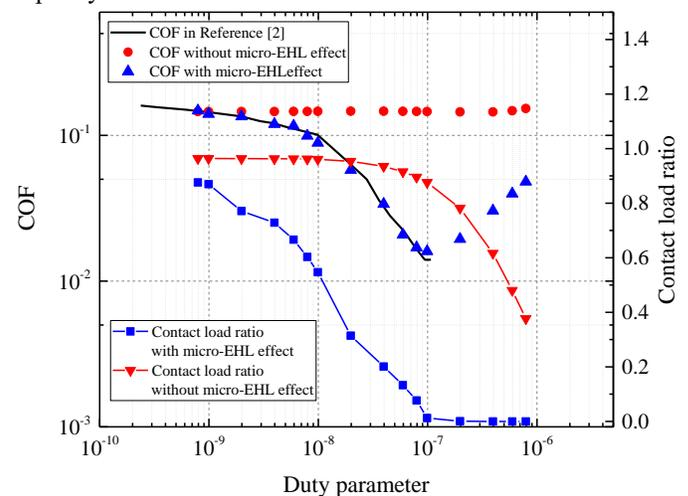
Fig.1 Comparison of simulated and experimental Stribeck curve and contact load ratio results with and without the micro-EHL effect at asperity scale
