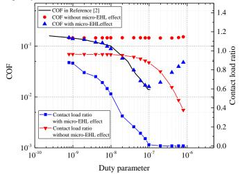
Fig.1 Comparison of simulated and experimental Stribeck curve and contact load ratio results with and without the micro-EHL effect at asperity scale
