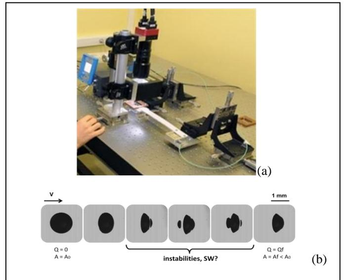
Fig.1 In-situ visualization tribometer (a). Evolution of the contact area morphology (in black) in a PDMS/Glass interface during shearing (b).
