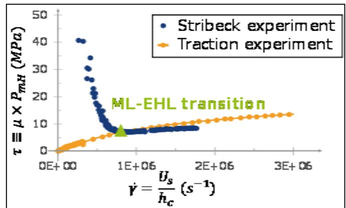
Fig.1 Stribeck and traction curves allowing to define the mixed-EHL transition (example with a low viscosity base oil: steel/steel, mean Hertz pressure 440MPa, Stribeck SRR 25%, inlet oil viscosity 23 mPa.s at 27°C)
