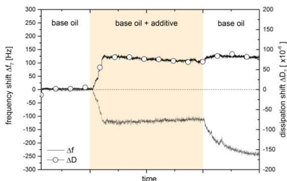
Fig.1 Exemplary frequency and dissipation shift from QCM-D tests: adsorption of friction modifier from mineral base oil
