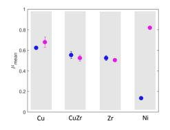
Figure 1 - Mean friction coefficient of AMAs at 2 different contact pressures: 310 MPa (Blue) and 680 MPa (Pink)
