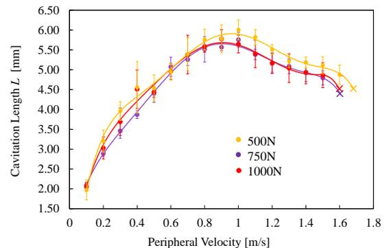
Figure1. Experimental cavitation length with peripheral velocity at each load
