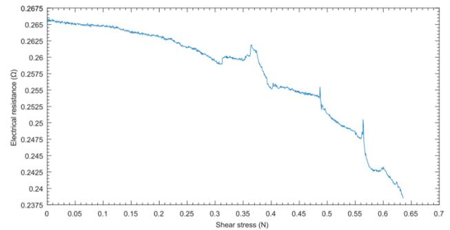
Fig. 2 Contact resistance vs. shear stress of an Al/Al interface
