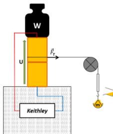
Fig.1 Experimental setup: metallic cylindrical samples in contact, undergoing a normal and a tangential stress. Voltage is measured at each end of the set during the shear increasing.
