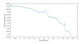
Fig. 2 Contact resistance vs. shear stress of an Al/Al interface
