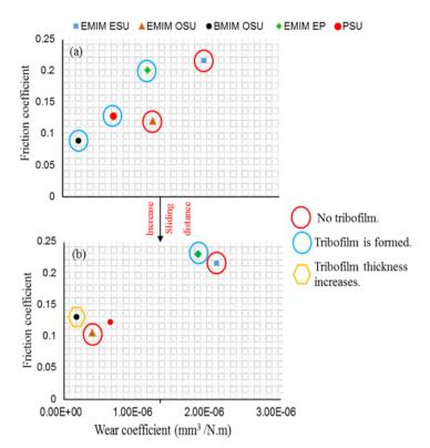
Fig.1 : The lubrication mechanism of ILs at various sliding distances.
