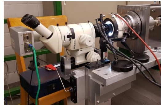
Fig.1: Optical radial lip seal test rig
