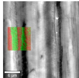
Fig.1 Overlay of the friction signal over the topography of the wear track; green region indicates lower friction
