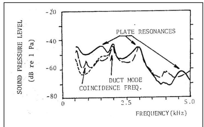
Figure 1. Measured (long dash), Modeled with radiation efficiency =1 (solid), Modeled with radiation efficiency estimated from theory (short dash)
