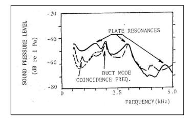
Figure 1. Measured (long dash), Modeled with radiation efficiency =1 (solid), Modeled with radiation efficiency estimated from theory (short dash)
