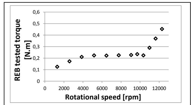
Fig.1: REB resistive torque
