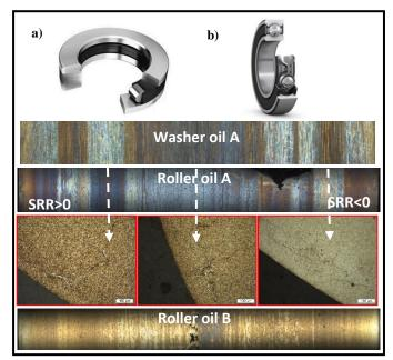
Figure 1 : Type of bearing tested, CRTBs (a), DGBBs (b) and typical WECs only observed for oil A and not B.
