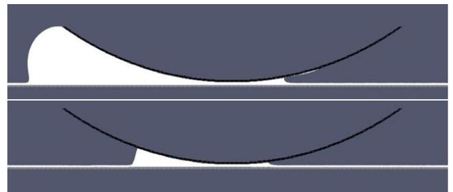
Fig. 2 Snapshots of hydrodynamic lubrication with sufficient (upper) and insufficient (lower) lubricant film, model geometry and condition are same with the Fig.3(a) of ref. [1].
