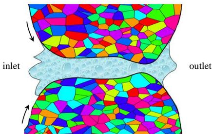
Fig.1 Schematic graph of an EHL lubricated conjunction with anisotropic material
