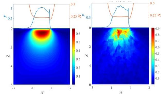
Fig.2 The influence of isotropy and polycrystalline anisotropy material on EHL pressure, film thickness and subsurface Von Mises stress distribution (Newtonian fluid,  $L=10, M=50$ )
