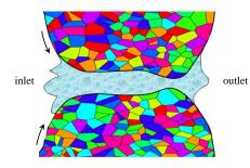
Fig.1 Schematic graph of an EHL lubricated conjunction with anisotropic material
