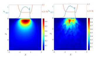
Fig.2 The influence of isotropy and polycrystalline anisotropy material on EHL pressure, film thickness and subsurface Von Mises stress distribution (Newtonian fluid, L=10, M=50)
