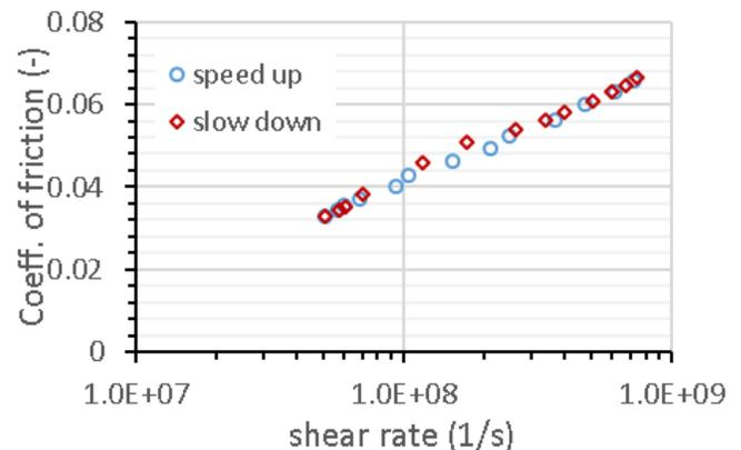
Fig.2 Friction data of measurement in Fig. 1
