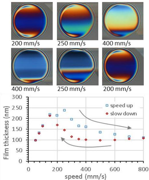
Fig.1 Film thickness and several interferograms from ramp up and down experiments.
