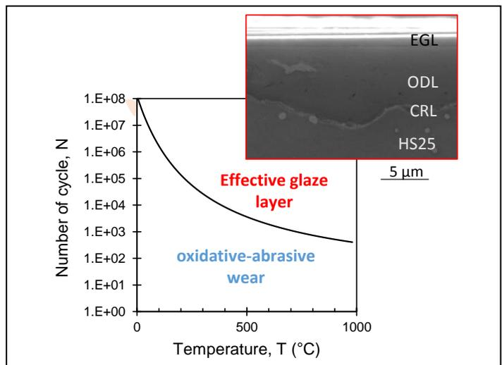
Fig.1 Prediction of the glaze layer formation and SEM observation of the high-temperature tribolayer
