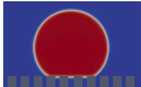
Fig. 1: Simulation of liquid (red) on a textured surface (gray)
