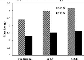
Fig.1 Mass loss as function of normal load
