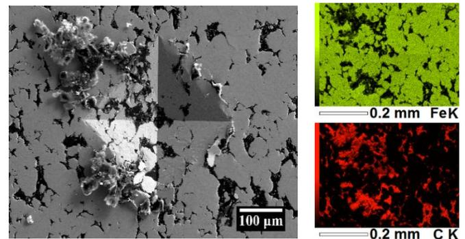
Fig.1 SEM and EDS images of graphite particles extrusion after Vickers indentation with a load of 10 kgf
