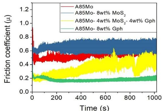
Fig.2. Friction coefficient of the sintered composites under dry sliding test at 20 N of applied load
