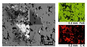
Fig.1 SEM and EDS images of graphite particles extrusion after Vickers indentation with a load of 10 kgf
