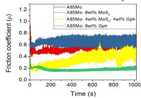
Fig.2. Friction coefficient of the sintered composites under dry sliding test at 20 N of applied load
