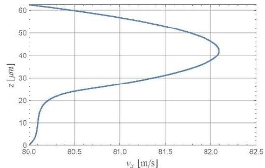
Fig.3 Typical oil velocity profile in rolling contact at a location of negative pressure gradient. Upper portion of the curve is pure oil, the lower portion is oil flow in thickener.
