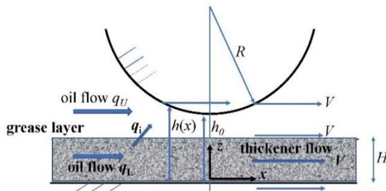
Fig.1 Schematic of grease layer in cylinder/plane rolling contact. The gap contains a lower grease layer (thickener plus oil) supplying an upper oil film.
