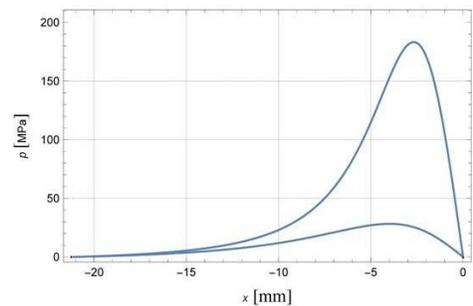
Fig.2 Pressure profiles in rolling contact, two cases. For the lower curve, the gap is pure oil; for the upper curve, a grease layer is present.
