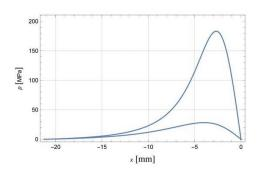
Fig.2 Pressure profiles in rolling contact, two cases. For the lower curve, the gap is pure oil; for the upper curve, a grease layer is present.
