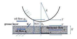
Fig.1 Schematic of grease layer in cylinder/plane rolling contact. The gap contains a lower grease layer (thickener plus oil) supplying an upper oil film.
