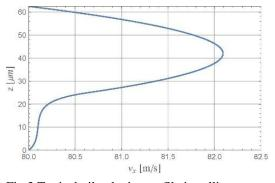
Fig.3 Typical oil velocity profile in rolling contact at a location of negative pressure gradient. Upper portion of the curve is pure oil, the lower portion is oil flow in thickener.
