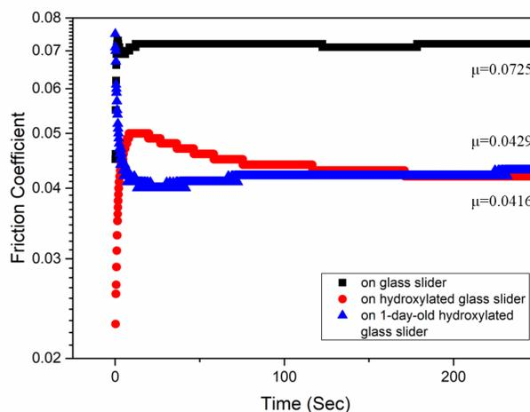
Fig.1 Friction coefficient as a function of time under lubrication between the PTFE ball and glass slider when PPE is used as a lubricant. Different colors stand for different conditions (black square for the plain glass slider, red dot for the fresh hydroxylated glass slider, blue triangle for the hydroxylated glass slider prepared one day before testing).
