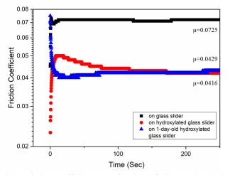
Fig.1 Friction coefficient as a function of time under lubrication between the PTFE ball and glass slider when PPE is used as a lubricant. Different colors stand for different conditions(black square for the plain glass slider, red dot for the fresh hydroxylated glass slider, blue triangle for the hydroxylated glass slider prepared one day before testing).
