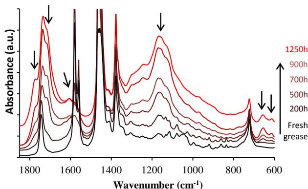
Fig.1. IR spectra of fresh grease oxidized from 200 to 1250h at 130 °C from 600 to 1800  $\text{cm}^{-1}$
