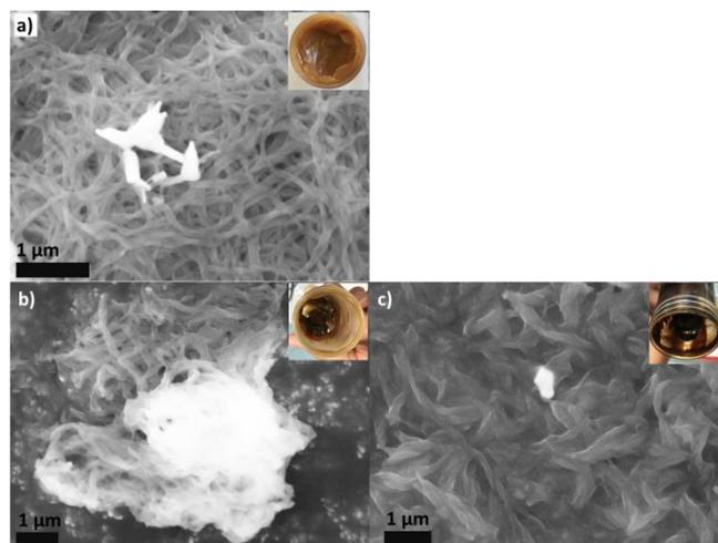
Fig. 3. SEM images of: a) fresh thickener, b) oxidized thickener c) sheared thickener
