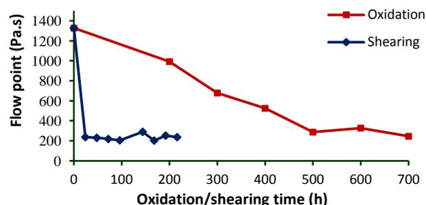
Fig. 2. Impact of churning time on fresh grease flow point
