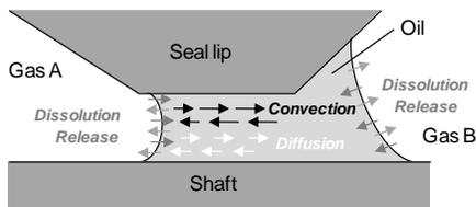
Fig.1 Gas transportation at seal lip
