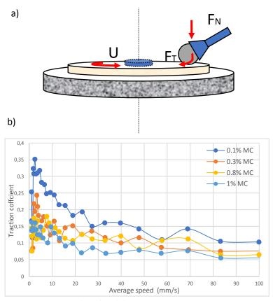
Fig.1 a) Schematic of Mini traction machine (MTM) b) coefficient of traction versus speed of 0.1-1% Methyl Cellulose.
