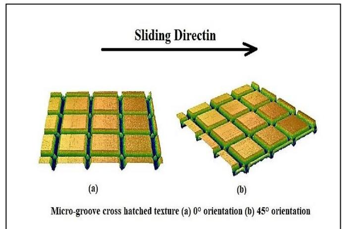
Fig.1 3D images of Micro-groove cross hatched texture with different orientations
