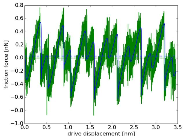
Fig.1 Friction force at 0 K (blue) and room temperature (green) obtained from a 1D PT-model with a periodic corrugation.
