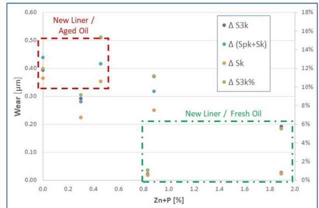
Figure 2- Liner wear and % of Zn+P found in the wear track.
