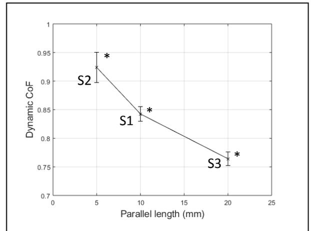
Fig.1 Relationship of rubber sample length and dynamic  $\mu$  of three different shapes of rubber
