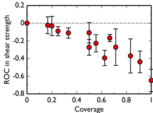
Fig. 1 Plots of ROC in interfacial shear strength against film coverage in patterned surfaces
