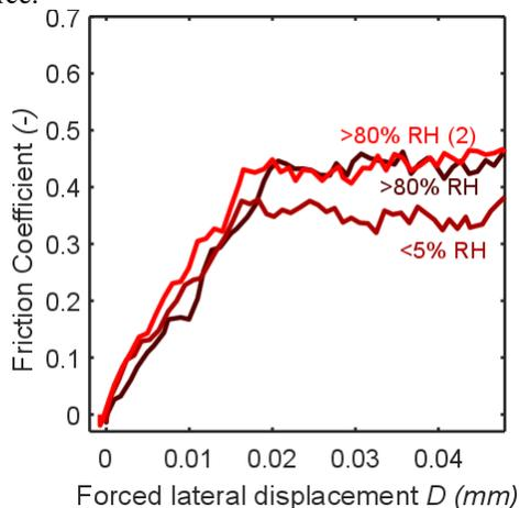
Fig.1 Friction coefficient measured at the interface between a rough SiC ball and a smooth Si wafer. The friction can be switched from high to low and back by changing the relative humidity of the surrounding air.
