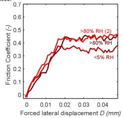
Fig.1 Friction coefficient measured at the interface between a rough SiC ball and a smooth Si wafer. The friction can be switched from high to low and back by changing the relative humidity of the surrounding air.
