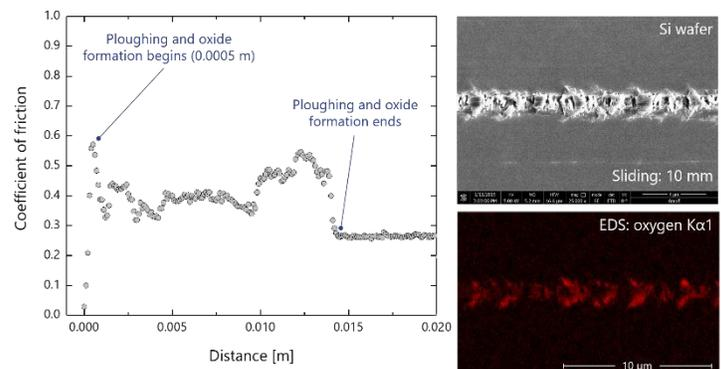
Fig.1 Coefficient of friction as a function of sliding distance for SiC-on-Si contacts. SEM image and corresponding EDS map illustrating ploughing and oxide formation at 10 mm sliding.
