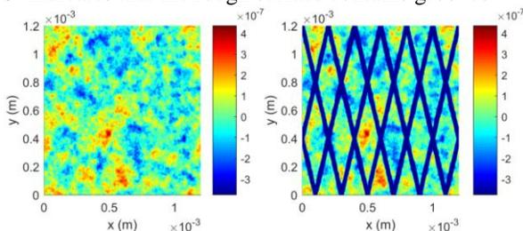
Fig.1 Cylinder liner surfaces: 'R' (left) and 'R+G' (right).
