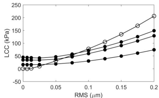
Fig.3 LCC as a function of the surface RMS roughness for 'R' (open dots) and for 'R+G' with a groove spacing of 0.1,0.2,0.3 mm bottom to top (closed dots).
