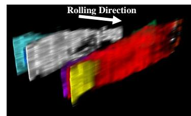
Fig.1 3D-model of HABs in ACBB inner ring
