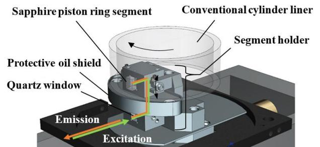
Fig. 1 Optical access in the rotational tribometer for oil-film visualization on a commercial liner surface.
