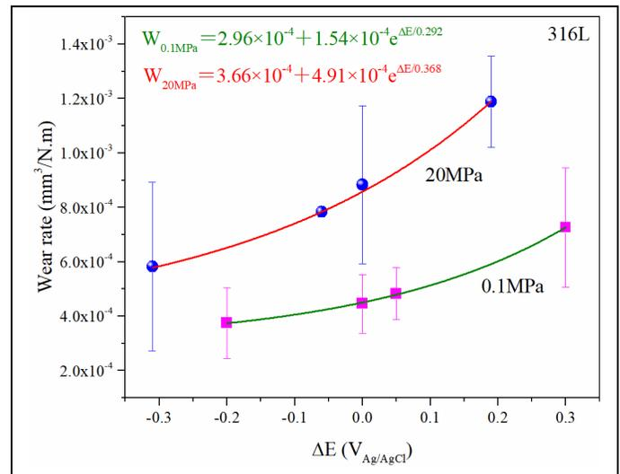
Fig.1 Dependence of wear rates of 316L stainless steel on the value of polarization at different hydrostatic pressures.
