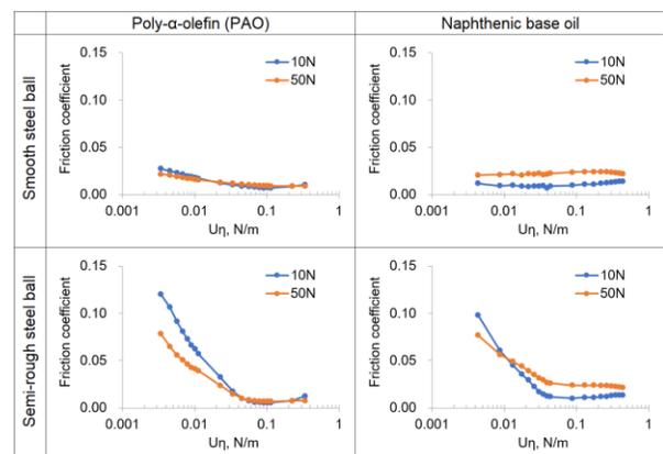
Fig.1 Friction coefficient as a function of  $U\eta$
