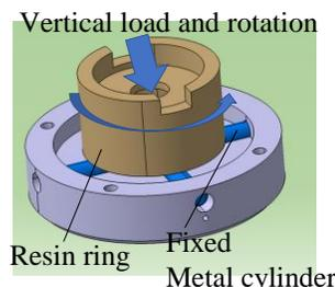
Fig.1 Schematic view of testing device
