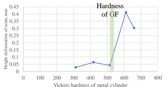
Fig.2 Relation between Vickers hardness of metallic cylinder and height deformation of resin ring reinforced by GF.
