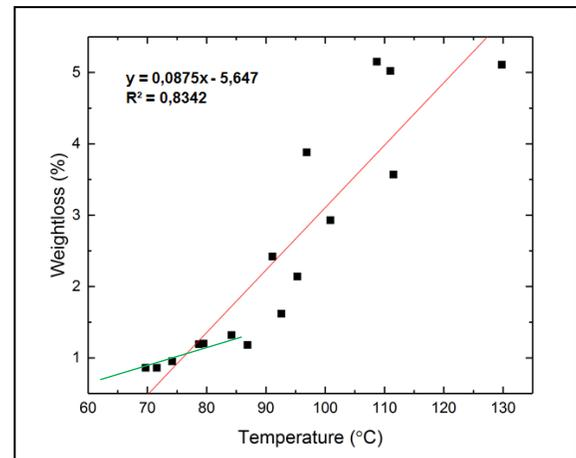
Fig.1 Effect of the pyrometer-measured contact temperature on the weight loss for an elastomeric coating (tests on a belt-pulley laboratory simulator)
