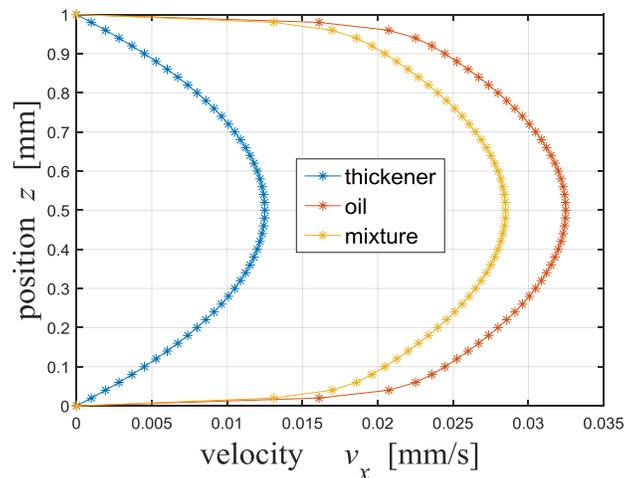
Fig.1 Velocity profiles in channel flow of grease, Darcy-Brinkman model
